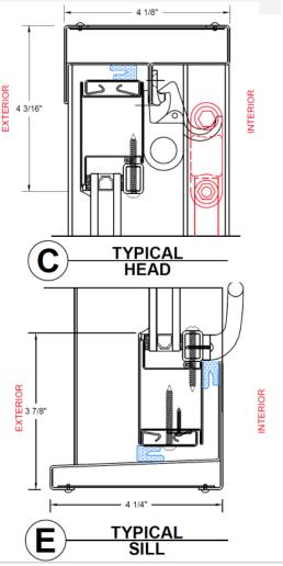
NOTE: This product is intended for use in locations requiring fire-protective rated openings.
